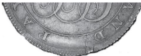
Fig. 5. Detail of the die flaw on the edge of *D&H: Middx 305*.
